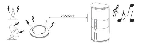
5. You should now be able to place the speakers freely from room to room without disruption. Should there is any disruption (signal cuts off or carries distortion), press the speaker's "AUTO TUNE" button to maximize the best reception.
