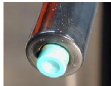
Tapping button reverses spindle direction
