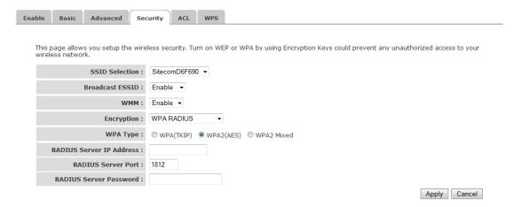
Wi-Fi Protected Access (WPA) is an advanced security standard. You can use an external RADIUS server to authenticate wireless stations and provide the session key to encrypt data during communication. It uses TKIP or CCMP (AES) to change the encryption key frequently. Press **Apply** when you are done.
