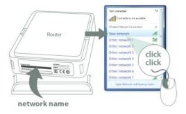
• Fill in the password for the wireless network. The correct password can be found on the sticker on the bottom of the router, or in the Network Details Folder.
