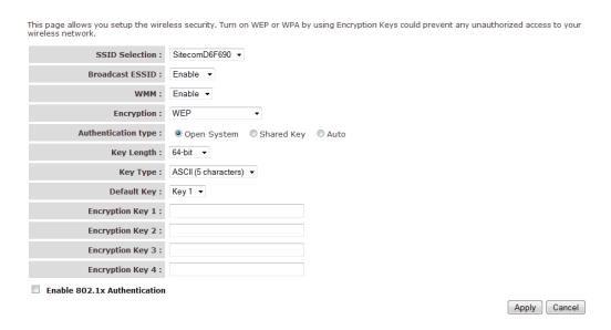
When you select 64-bit or 128-bit WEP key, you have to enter WEP keys to encrypt data. You can generate the key by yourself and enter it. You can enter four WEP keys and select one of them as a default key. Then the router can receive any packets encrypted by one of the four keys.
