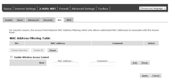
This wireless router supports MAC Address Control, which prevents unauthorized clients from accessing your wireless network.
