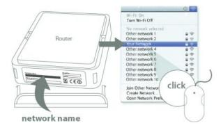
• Fill in the password for the wireless network. The correct password can be found on the sticker on the bottom of the router, or in the Network Details Folder.
