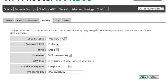
Wi-Fi Protected Access (WPA) is an advanced security standard. You can use a preshared key to authenticate wireless stations and encrypt data during communication. It uses TKIP or CCMP (AES) to change the encryption key frequently, so the encryption key is not easy to be cracked by hackers. This is the best security available.
