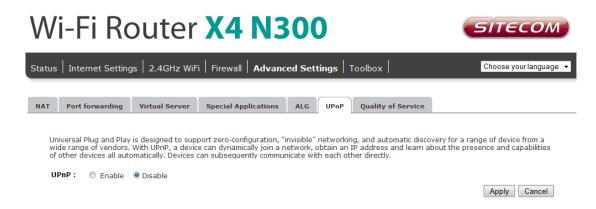
**UPnP Feature**: You can enable or Disable the UPnP feature here. After you enable the UPnP feature, all client systems that support UPnP, like Windows XP, can discover this router automatically and access the Internet through this router without having to configure anything. The NAT Traversal function provided by UPnP can let applications that support UPnP connect to the internet without having to configure the virtual server sections.
