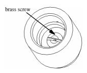
You can also adjust the brass screw inside the XM-CHARGER. In this case, you need to use screw driver and counter-clockwise to turn the brass screw up.
