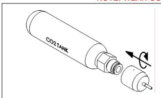
Step 01: Attach XM-CHARGER onto your CO2 tank.
