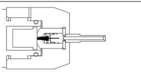
Step 02: There should be CO2 output. If not, please follow the steps below: The CO2 tank valve is not pushed by the XM-CHARGER's brass screw. Not all tank valves are built the same and you need to do with the height of the pin located at the center of the valve.
