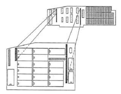
Press the pins gently but firmly into the sockets until they are fully seated. (Even when it's fully seated there may still be some of the pin showing between the connectors, so don't press too hard!) Now, re-install the expanded RamWorks following the installation instructions in your user's manual
