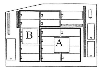
It is extremely important to insert the Expander's memory chips properly. The illustration shows the correct orientation of the RAM chips and which memory chip sockets are allocated to each block on the 2 Meg+ Expander. Note the position of the notch (or dot on some chips). Each RAM chip should have all legs fully seated in the socket and in the correct position.
