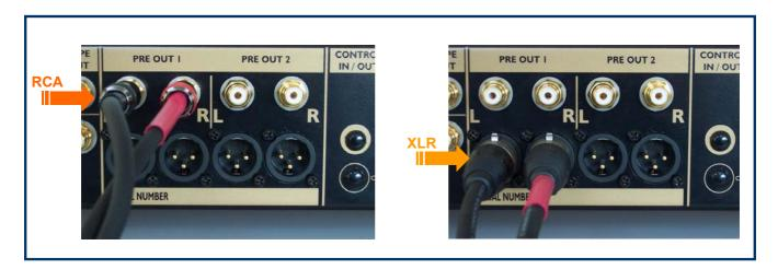
All four outputs are always active and can be utilised in multi-amp configurations.
