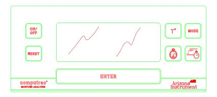
The front panel LCD consists of three separate fields and easy-to-understand symbols. Test information such as the sample's current weight or the computed moisture result, as well as the elapsed test time and the test temperature are displayed. As an added convenience, the display includes a linear range indicator for the precise control of the beginning sample weight.
