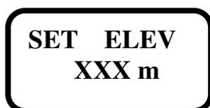
Offered is the elevation which was used during previous flight. If the glider is situated always on the same airfield this figure should be only checked and simple confirmed with **escape**. If the figures don't match field elevation a **correction** should be done. After field elevation input also the altitude reading of **Vario unit will change**, to match field elevation set in LX 166.
