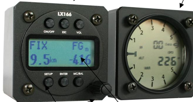
Vario unit doesn't have any controls and is completely under LX 166 Main unit control. LX 166 Main unit has one **multifunctional rotary switch**, six **push buttons** and a **graphic display**.
