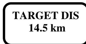
This input isn't active after LX 166 is coupled with GPS. The distance is replaced with GPS status data.
