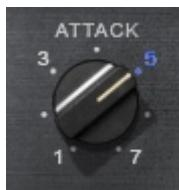
**Range:** 1 (slowest - 1 millisecond) to 7 (fastest - less than 50 microseconds) in 0.0x steps
