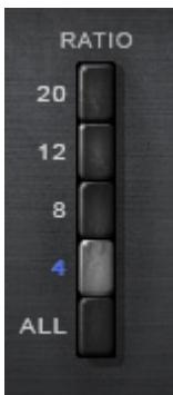
Like many compressors, the higher the ratio, the higher the threshold. For example, at a ratio of 20:1, the threshold point is -12 dBFS, meaning that every peak which passes -12dBFS will be compressed at a 20:1 ratio. When ratio is set to 4:1, the threshold drops to -18dBFS, meaning that every peak which passes -18dBFS will be compressed at a ratio of 4:1. This, therefore, results in “more” compression, despite the lower ratio.
