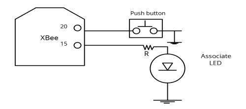
To support the Commissioning Pushbutton and its associated LED functions, connect a pushbutton and an LED to device pins 20 and 15 respectively.
