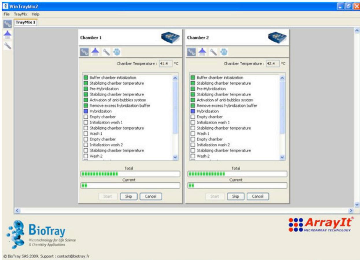
Hybridization proceeds at set time and temperature, with constant mixing.
