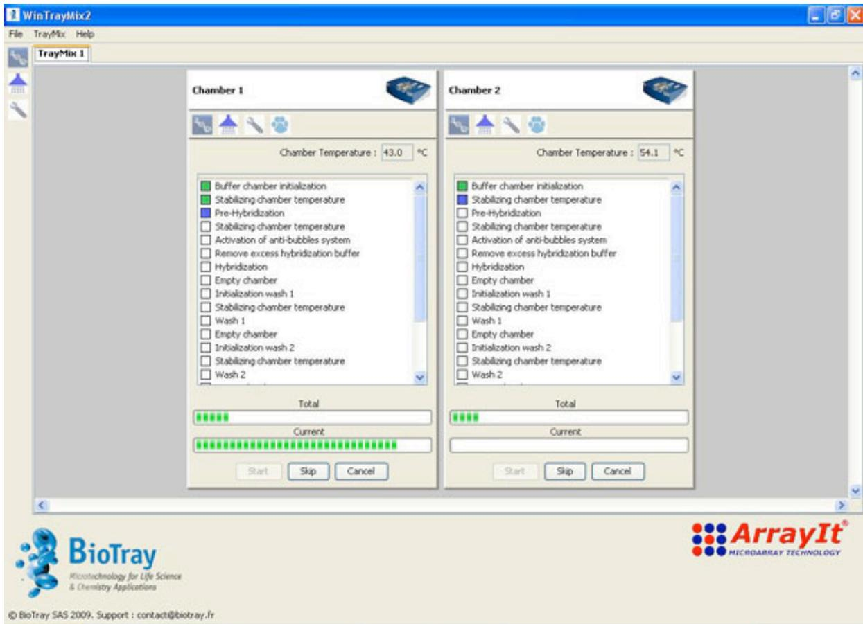
Programmed Pre-hybridization Program Starts, is useful to pre-hybridization to get the microarray at proper temperature and to wet the microarray prior to adding the labeled sample.
