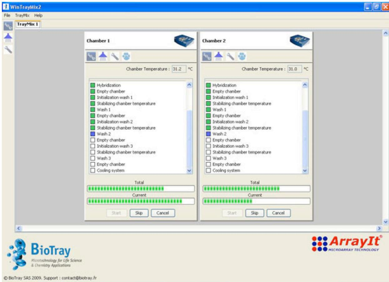
Wash steps proceed automatically based on set program parameters.
