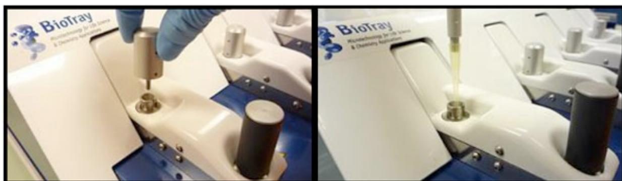
Once the system is programmed and the microarray substrate slides are in place on the platform, the system automatically delivers solutions into the hybridization chambers. The 50  $\mu$ l hybridization chambers are sealed using gaskets located on the upper portion of the lids that each microarray when they are in the closed and locked position.
