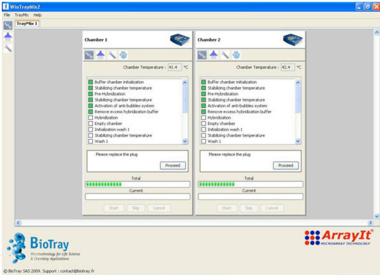
Depending on the volume of injection, the mixing loop automatically compensates for the volume injected for hybridization.
