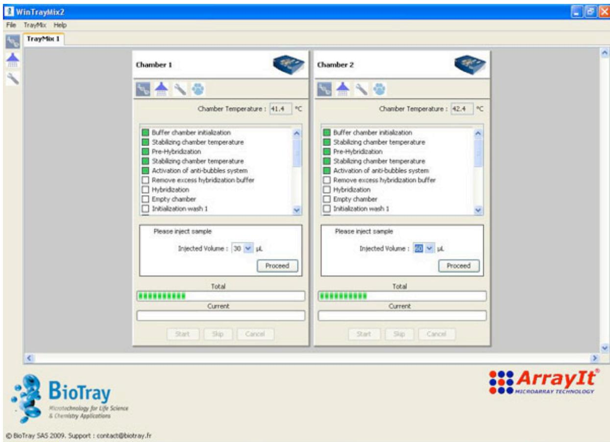
Injecting the sample is done with a volume of 30 µl or 60 µl, set volume, inject sample and click proceed.
