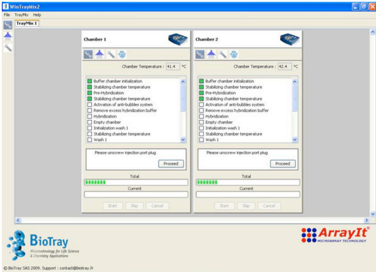
After Pre-hybridization is completed, temperature is stabilized, the next step is to remove air bubbles for the chaotic advection mixing loop.
