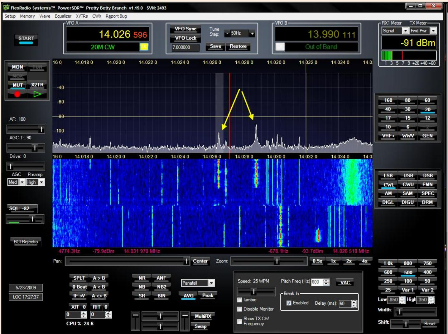
PowerSDR's use is not limited to the Flex radios. For example, I use PowerSDR to provide bandscope functions to my FT2000 – as shown in the picture above. Many of the convenience functions of PowerSDR work with the 2K - including adjustable bandwidth display, signal decoding, filtering and noise reduction, as well as mouse-click instant QSY.
