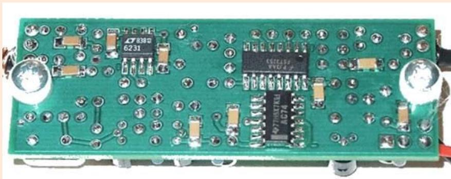
This SRII is tuned for the 10.55mhz IF of a FT-2000 and provides bandscope service. The displayed bandwidth and sensitivity (MDS) depends on the sound card it's matched with. In my application, the bandscope covers about a 100khz spectrum, and the minimum observable signal is better than -117dbm.
