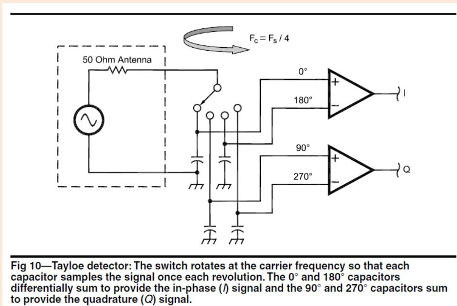
Fig 10—Tayloe detector: The switch rotates at the carrier frequency so that each capacitor samples the signal once each revolution. The 0° and 180° capacitors differentially sum to provide the in-phase (I) signal and the 90° and 270° capacitors sum to provide the quadrature (Q) signal.
