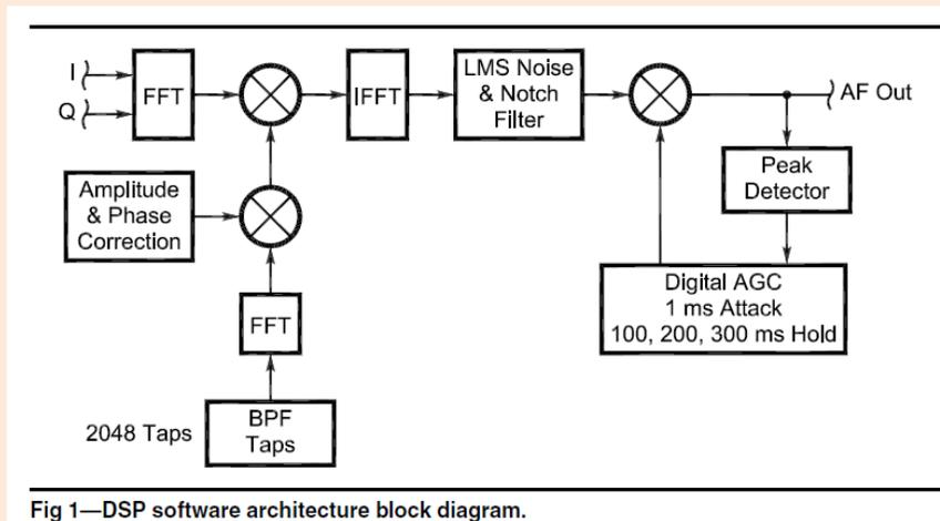
Fig 1—DSP software architecture block diagram.
