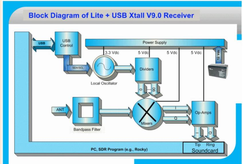
The Softrock v9 schematic here is very similar to the SR2:
