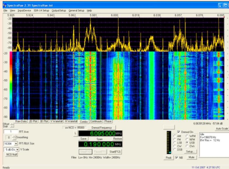
Rocky, by Alex VE3NEA of CW Skimmer fame. Rocky is a powerful program with a simple interface suitable for SDR hardware that is receive and transmit capable as well as for bandscope applications:
