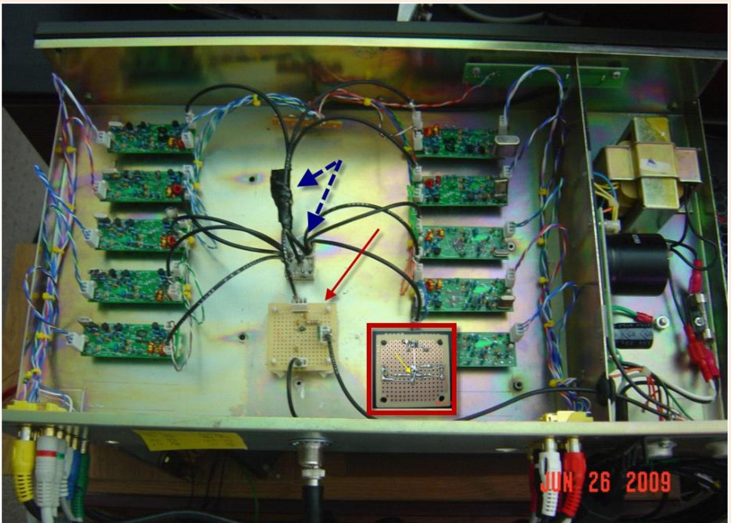
The output of the preamp is fed into an 8-way Mini Circuits splitter – one output leg of the 8-way is further split out into 3 additional lines serving the 160/80/40m bands. The 2<sup>nd</sup> series splitter adds an additional 6db or so of insertion loss - but given the high band noise levels encountered on these bands, the impact on sensitivity is insignificant.
