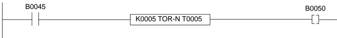
The internal coil, B45, is defined as the input to the TON-R timer, T5, which is a 10 msec base timer. The output of the timer is B50. K5 in the first cell of the timer block will give a delay of 5 x 10 msec = 50 msec. The output bit, B50, will turn on after 50 msec.
