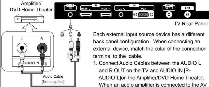
Each external input source device has a different back panel configuration. When connecting an external device, match the color of the connection terminal to the cable.
