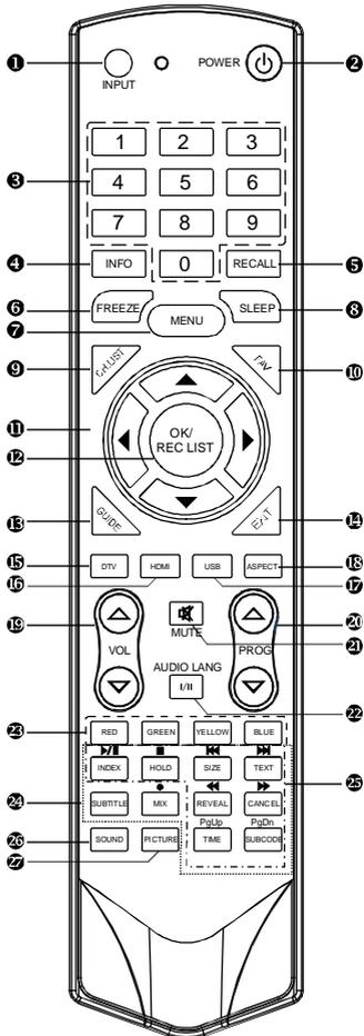
1. **INPUT:** This button is used to switch among different sources: DTV,ATV, AV1, AV2, AV3, Component, PC RGB, HDMI1, HDMI2, HDMI3, HDMI4, USB.
