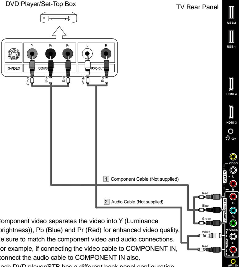
Component video separates the video into Y (Luminance (brightness)), Pb (Blue) and Pr (Red) for enhanced video quality. Be sure to match the component video and audio connections. For example, if connecting the video cable to COMPONENT IN, connect the audio cable to COMPONENT IN also.
