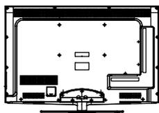
Thread hole size – M8 x 10 depth (TV mounting screw size) on the TV.
