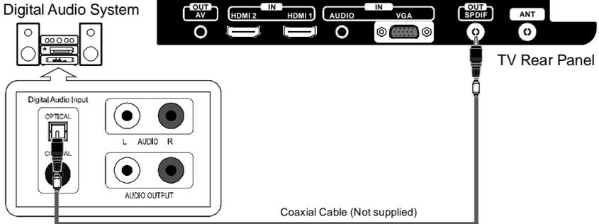
5.1 CH audio is possible when the TV is connected to an external device supporting 5.1 CH.
