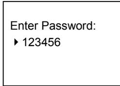
3. Press “◀” or “▶” to select the number of password digits. Enter the password digit by digit using “▲” or “▼”. Press “ENT” to confirm and enter the parameter setting submenu.
