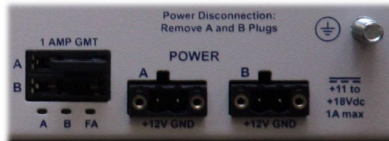
Fig. 5.2 The Trap48 RA's power inputs
