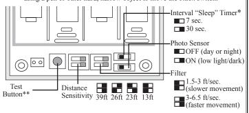
\*After detecting motion, the sensor can "sleep" for either 7 or 30 seconds, allowing an object to pass through the field of vision before setting the alarm off again.
