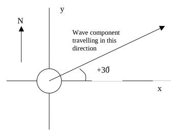
Orientation of direction relative to coordinate system for instrument layout and velocity components. With the compass orientation shown, the x axis direction is  $90^{\circ}$  in the file header.
