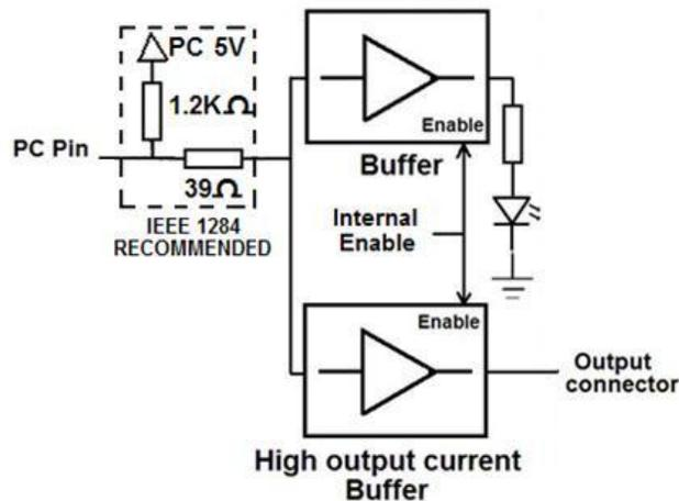
Simplified functional block diagram for the outputs 2-9
