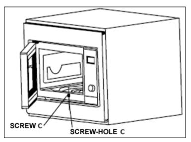
Open the microwave door and locate screw-hole C. Use screw C to fix the microwave oven to the housing unit. A screw cover is provided to cover the screw cap.
