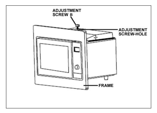
• Fit adjustment screw B into the adjustment screw-hole on the top of the microwave. Adjustment screw B should not be fully tightened at this stage.
