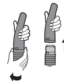
If cleaning tools were in use, check cleaning tool and extension tube first. Next check hose handgrip; to remove grip ribbed ring as shown, turn in direction of arrow and ease apart.
