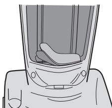
Remove bag door and lift out filter.
