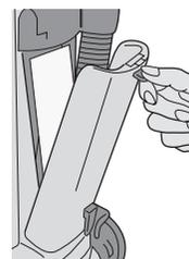
Press down on latch and remove the exhaust filter cover.
