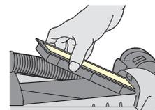
Lift out the exhaust filter.
