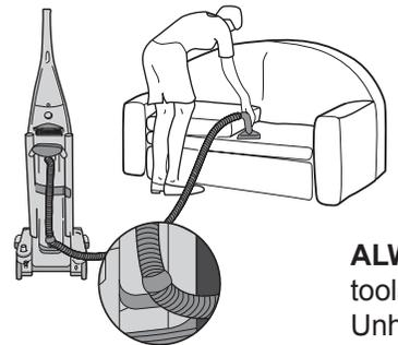
**ALWAYS** attach hose retainer to hook when using cleaning tools.
