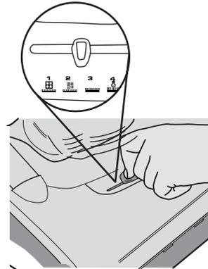
Ensure that the cleaner is in the upright (parked) position and move the selector to the required setting for the carpet type or floor covering.
