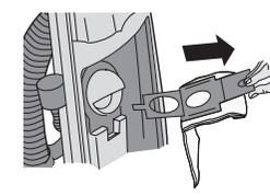
Slide bag from bag collar retainer by pulling on stiff cardboard at top of the bag collar. A shutter will automatically seal off bag opening.
