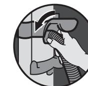
To check the hose, stretch it to full length and switch on the cleaner; the suction will dislodge most obstructions. If this is unsuccessful, switch off and unplug the cleaner. Remove the hose by turning it anti-clockwise as shown. Detach hose and remove blockage.
