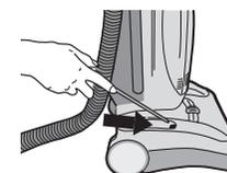
2. Check for a blockage in hose socket. Use a piece of wire or a blunt flexible rod to remove any obstructions.
