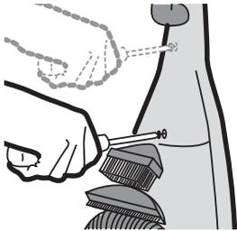
Insert handle into body of cleaner. Slide into position.
