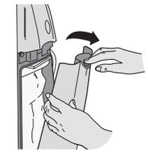
Press down on the door release pad and remove door.
