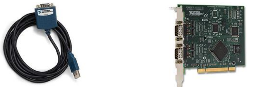
Figure 1: Hardware options for STIM210 evaluation kits (USB cable or PCI card)
