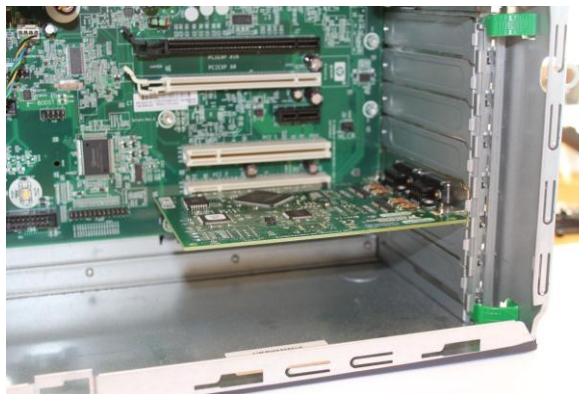
Figure 3: Stationary PC with STIM210 EVK PCI card
