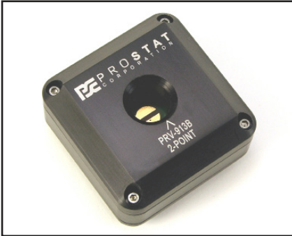
Figure 4: PRV-913B Dual Verification Fixture
