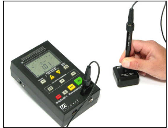
Figure 9: Insert PRF-912B Fixture into PRV-913B Verifier and Measure Verifier Resistance
