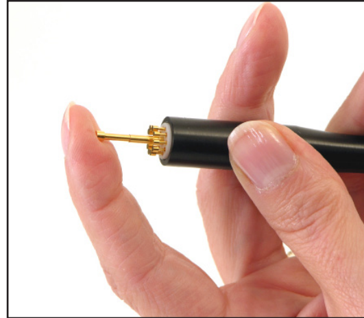
Figure 13: Insert Test Probe into its Socket and Press Firmly to fully seat
