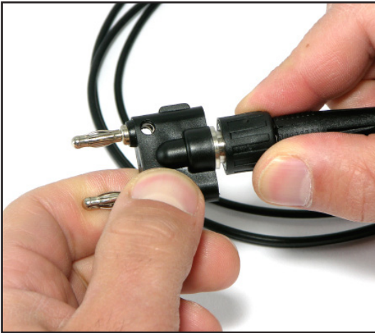
Figure 6: Connect Cable to Banana Converter
