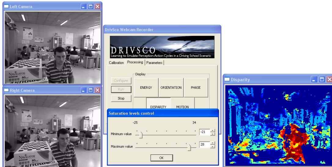
Fig. 1. Example of disparity processing. The saturation level control is available for change the colormap application visualization. The colormap in the case of the disparity shows closer objects with warm colors and farther ones with cold colors.
