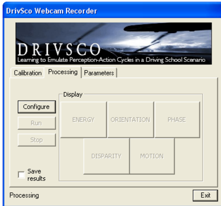
Fig. A.14. Processing Tab. It is the interface between the device board and the host computer. In this tab you select the processing which is going to be shown and stop this processing. The results can be saved.
