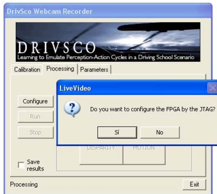
Fig. A.15. Example of use of the application. After clicking 'Configure' button, you can decide if the device is going to be programmed by the JTAG or throughout its PLX.
