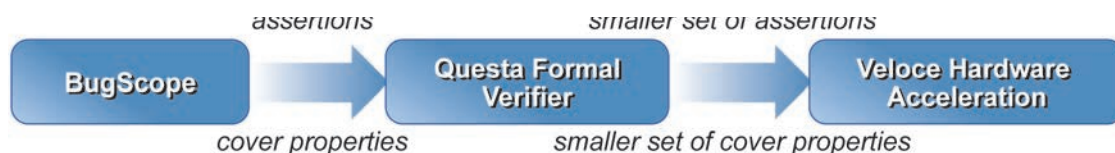
Figure 3 Assertion Synthesis Driven Hardware Acceleration Flow
