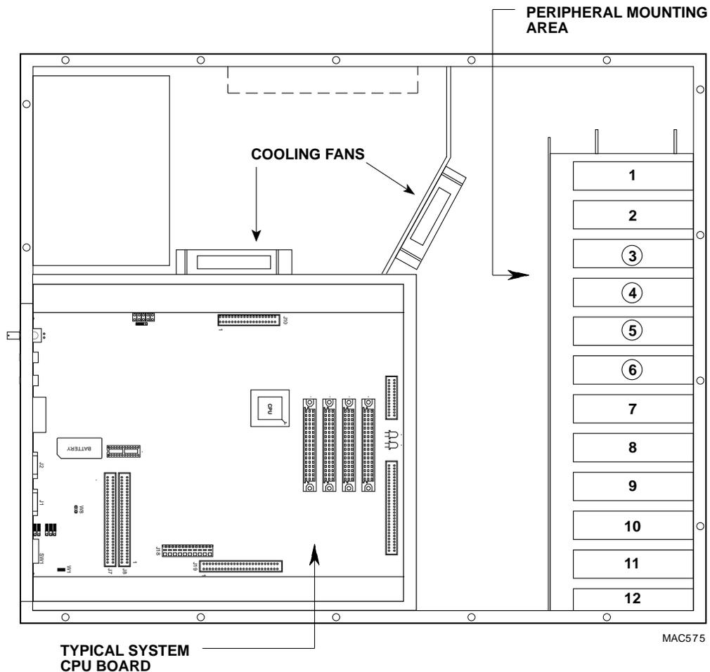
**Figure E-1 — SBC Peripheral Mounting Area**
