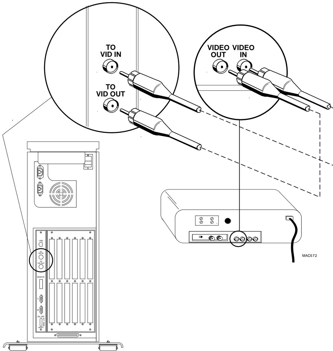
**Figure 2-7. Connecting a Video Cassette Recorder**
