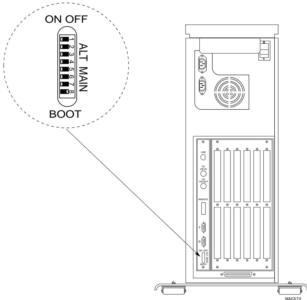
**Figure 2-1. Boot ID Switch Location**
