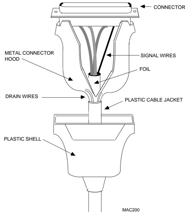
**Figure B-1. Shielding a Cable**
