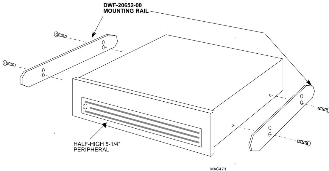
**Figure E-3 — Attaching Mounting Rails to Peripheral**
