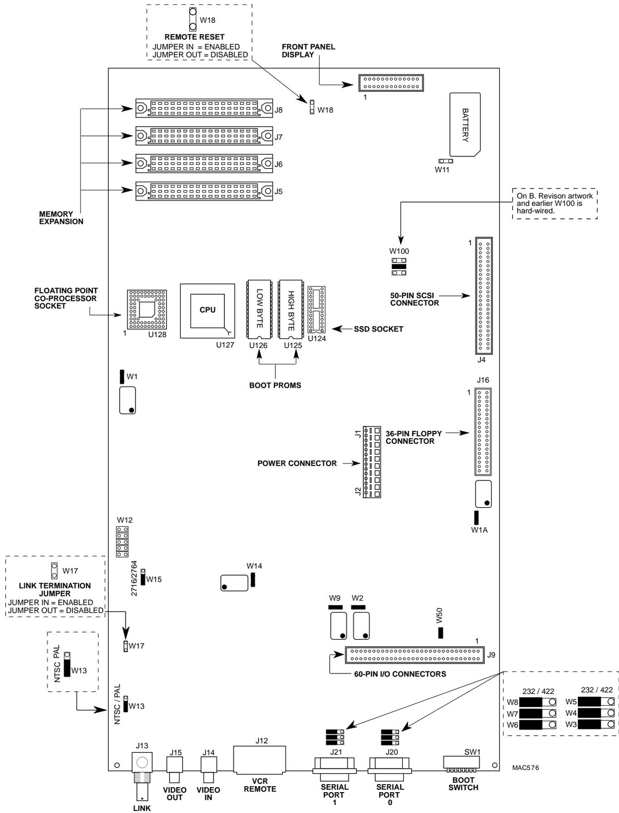
Figure G-1. Option Locations on the Main Logic Board
