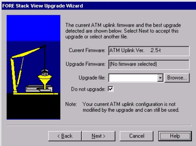
6. Make sure the **Do not upgrade** option has been selected and click **Next**. The FORE Stack View software will launch a TFTP server utility, perform the upgrade, and reset the switch.
