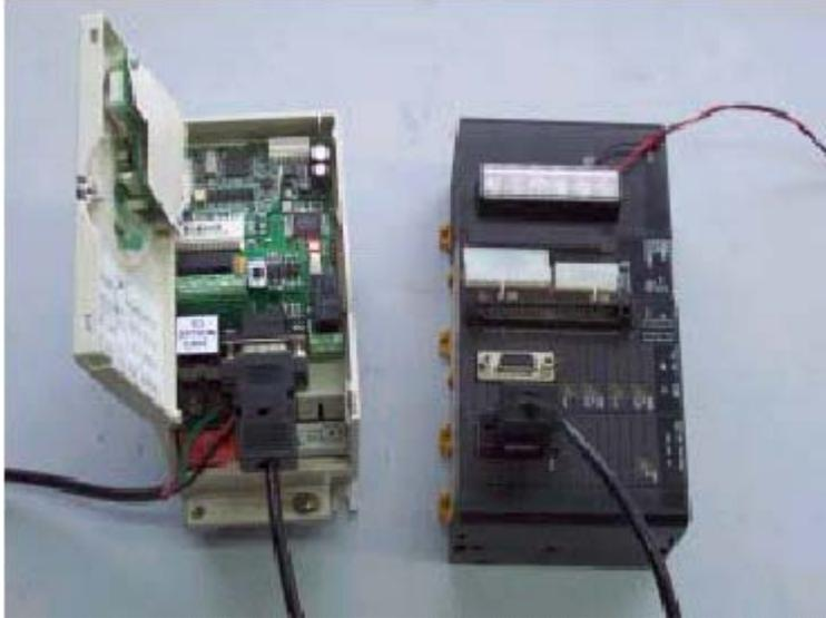
2. Toshiba Option unit can be connected to Profibus Option Card on Option Port.
