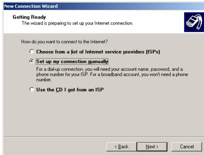
**Picture 19: Way of setting up a new connection**
