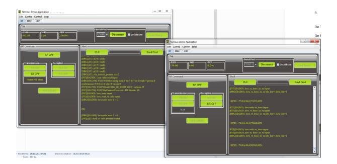
Note that, the reference ID in Rx mode is saved when module received his first frame. Remember this if you have problem during demo with LoRa interferences around or if you want to test 2 demos in parallel.
