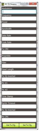
A simple couple of button to get the actual configuration and set the wanted configuration.
