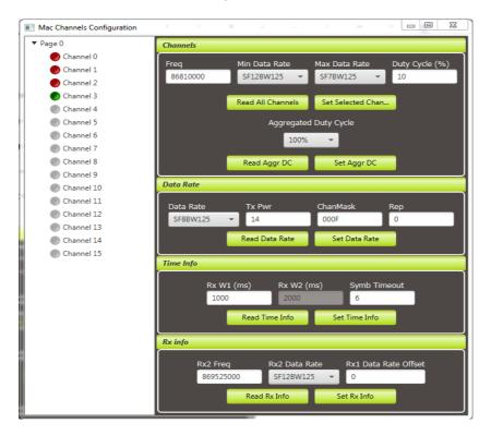
If you select a channel in the tree, the channel information is described in Channels part. Channel's frequency, data rate range and duty cycle information. Plus, the Aggregated Duty Cycle.
