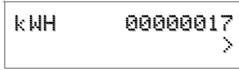
Fig. 12. The Class 100 kWh meter displays readings in whole numbers, there are no decimals.
