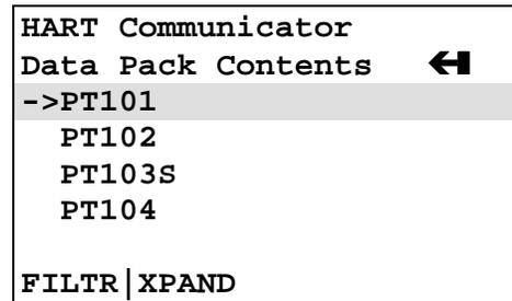
Sort allows unique device configurations to be grouped and displayed by Tag, Descriptor, or user-assigned Name.
