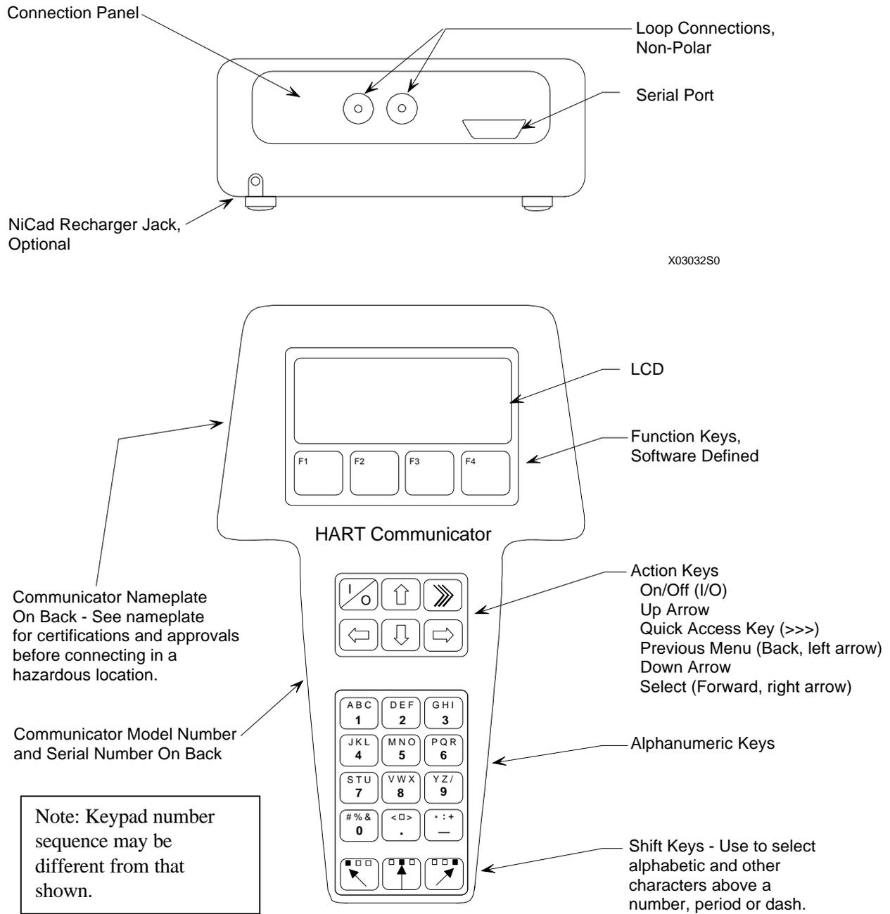
**FIGURE 2-1 Model 275 Universal HART Communicator**
