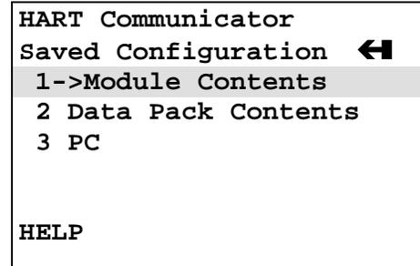
The Module Contents menu, which lists the configurations currently stored in the Memory Module, is shown at right. The Data Pack menu is similar. Both give the user several options for handling and viewing configuration data, as explained below.
