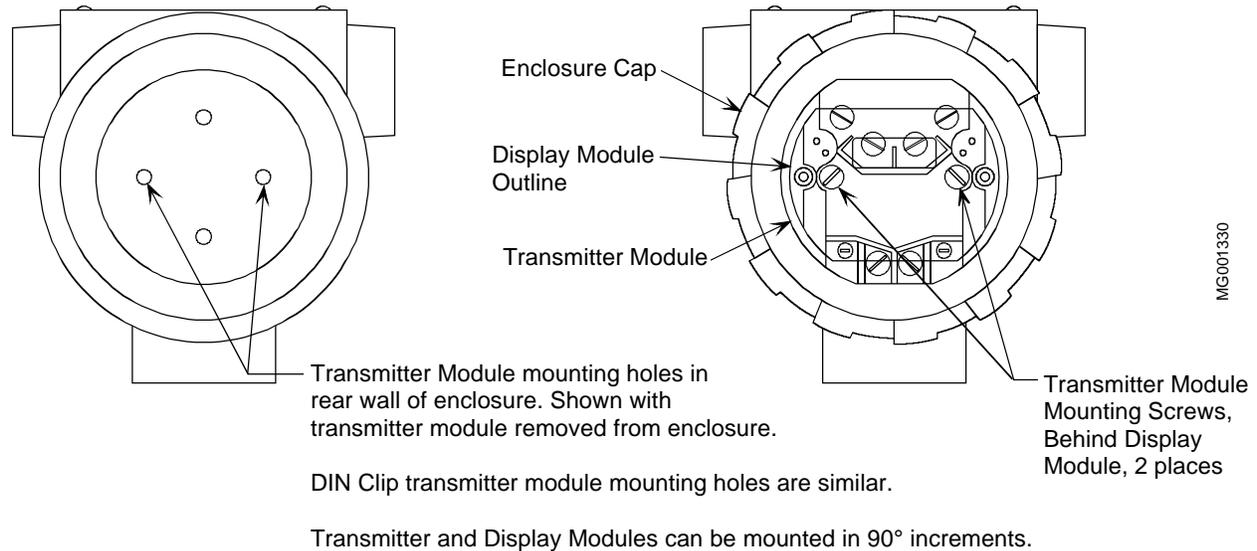
**FIGURE 4-9 Rotating a SmartDisplay or LCD Display (Model 343F Shown)**
