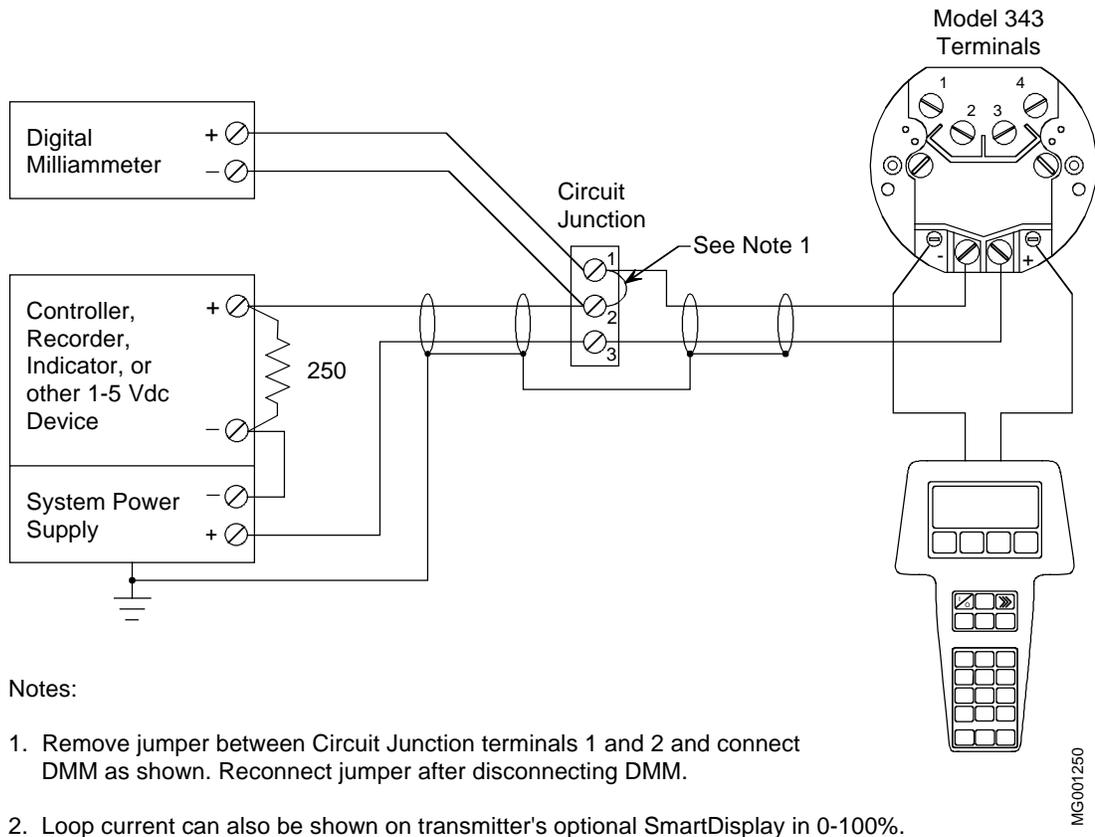
**FIGURE 3-2 Field Test Connections**
