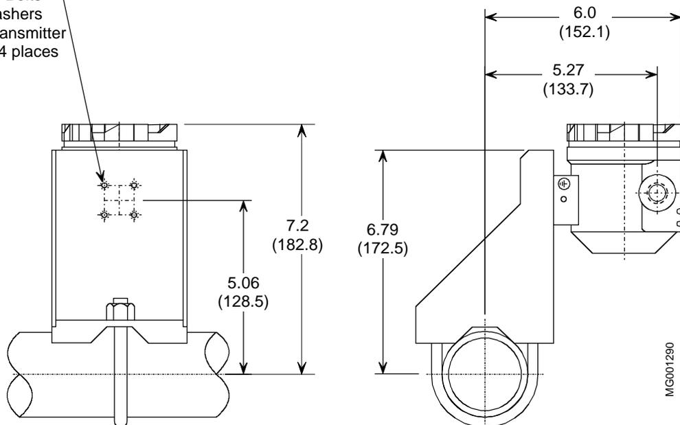
FIGURE 4-5 Dimensions, Model 343 on a Universal Mounting Bracket
