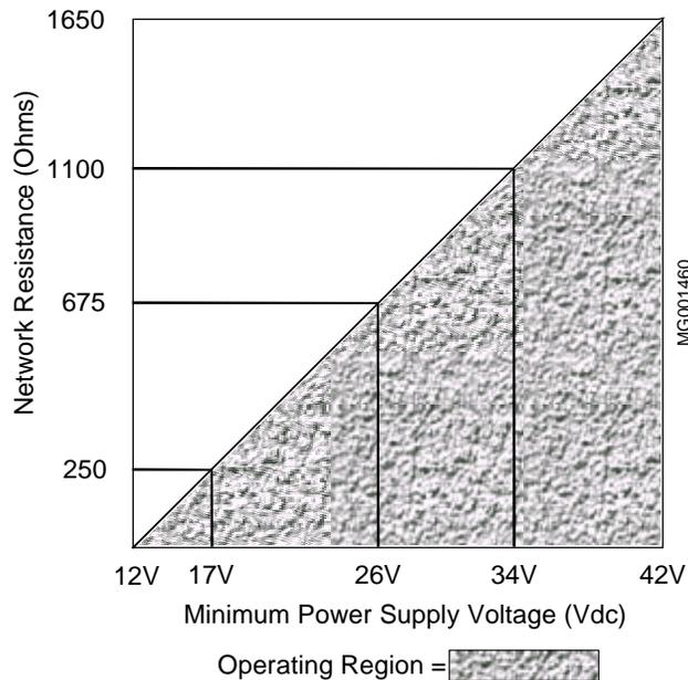
**FIGURE 4-4 Supply Voltage Versus Network Resistance**
