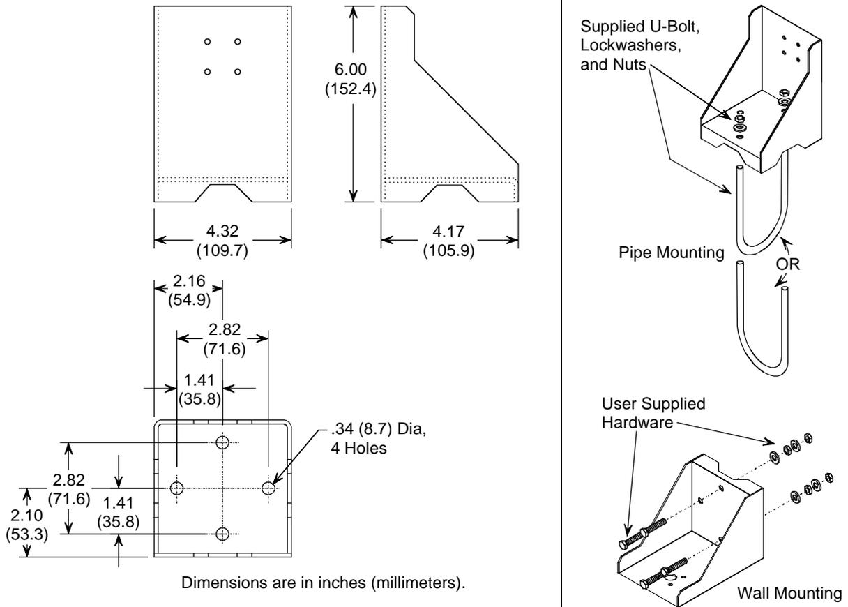
Use 1/4"-20 Bolts and Lockwashers to Mount Transmitter to Bracket, 4 places
