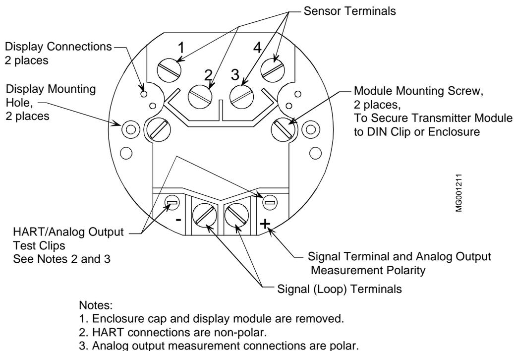
**FIGURE 1-2 Terminal Connections**
