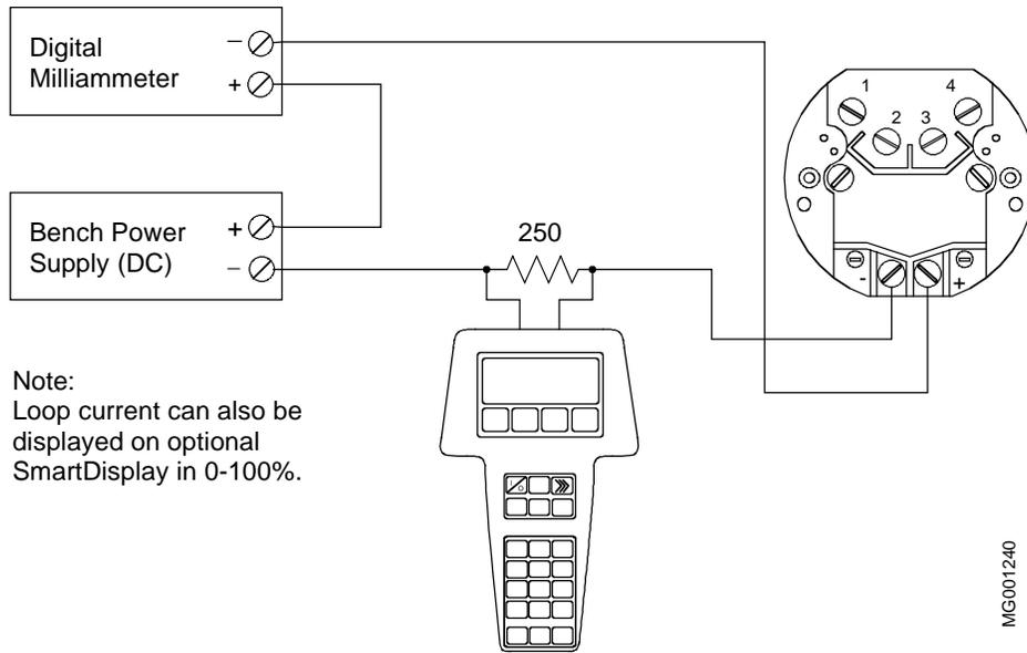
**FIGURE 3-1 Bench Test Connections**
