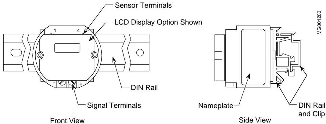
Model 343F - mount the transmitter as described in Section 4.4.1, 4.4.2, or 4.4.3.
