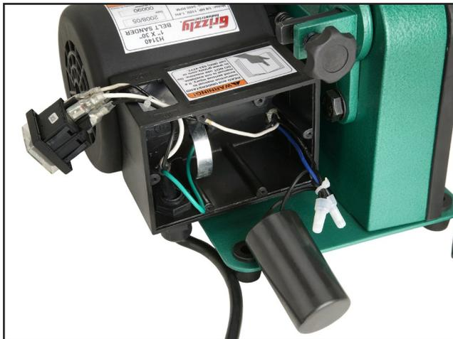
Figure 22. H3140 wiring.
