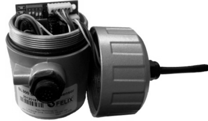
Figure 7 Dip switches are accessible for the required setting and calibration
