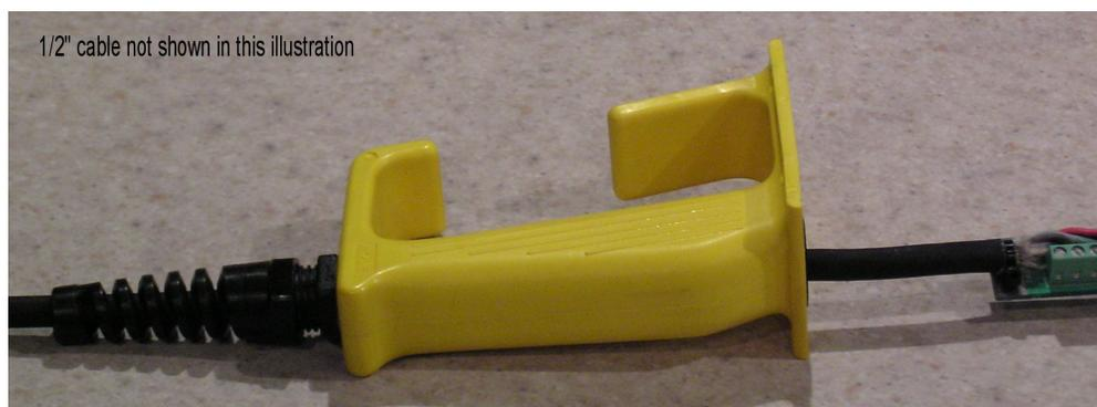
5) Cut of the tie-wrap and disconnect all the wires by loosening the screws at each terminal. Pull the cable out of the handle.
