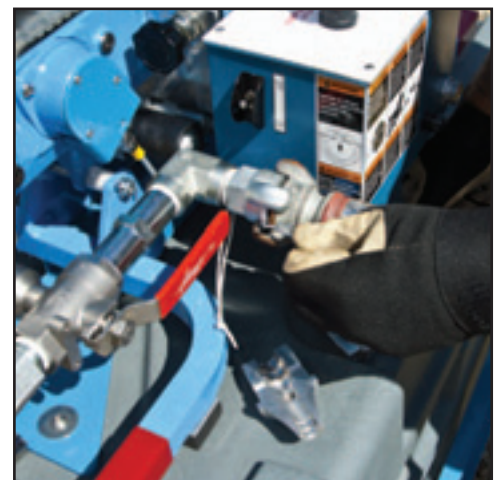
Figure 31. Installing Air Hose with Safety Clips
