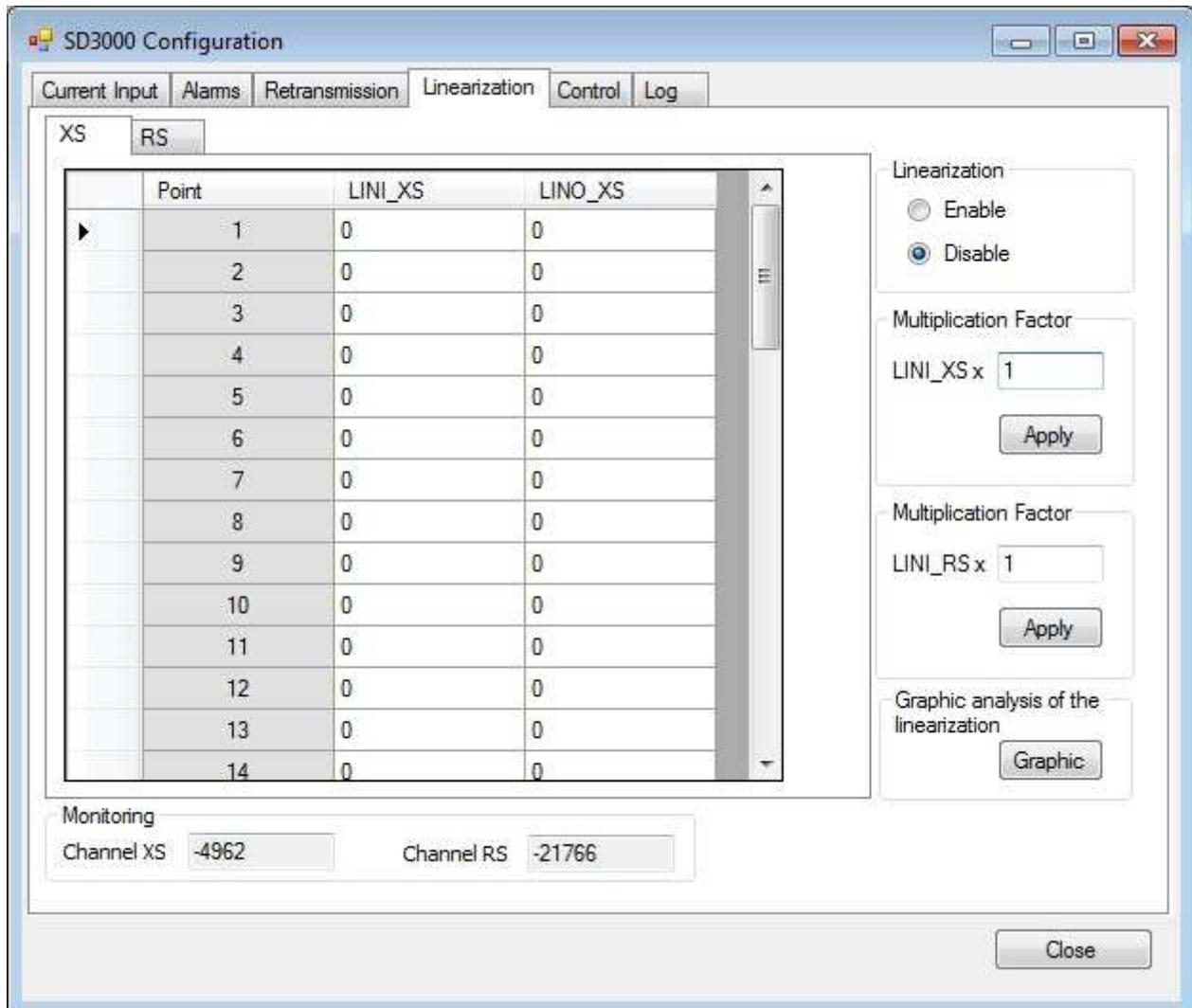
The SD-3000 has 2 linearization tables (XS and RS), with 50 points each. Linearization is enabled when bit 1 from the SD-3000 control register (address 40035) is set.
