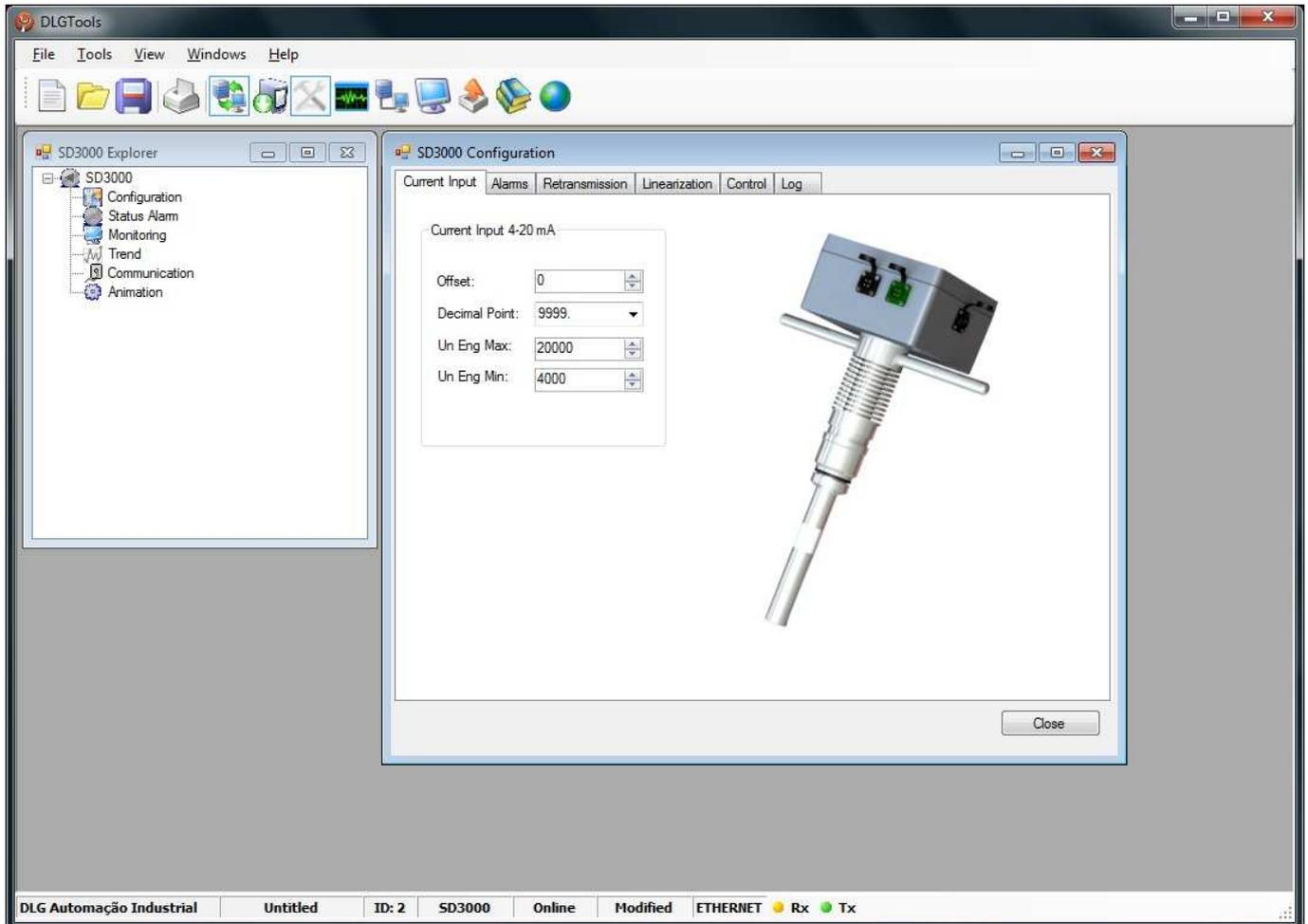
In the configuration screen it is possible to parameterize all SD-3000 registers.
