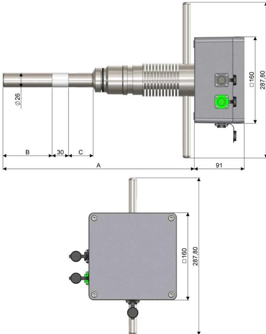
Figure 1 – Scaling mount (dimensions in mm)
