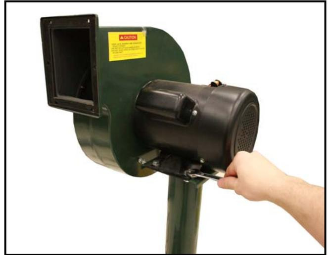
*Attaching Motor/Impeller to the Post Stand*
