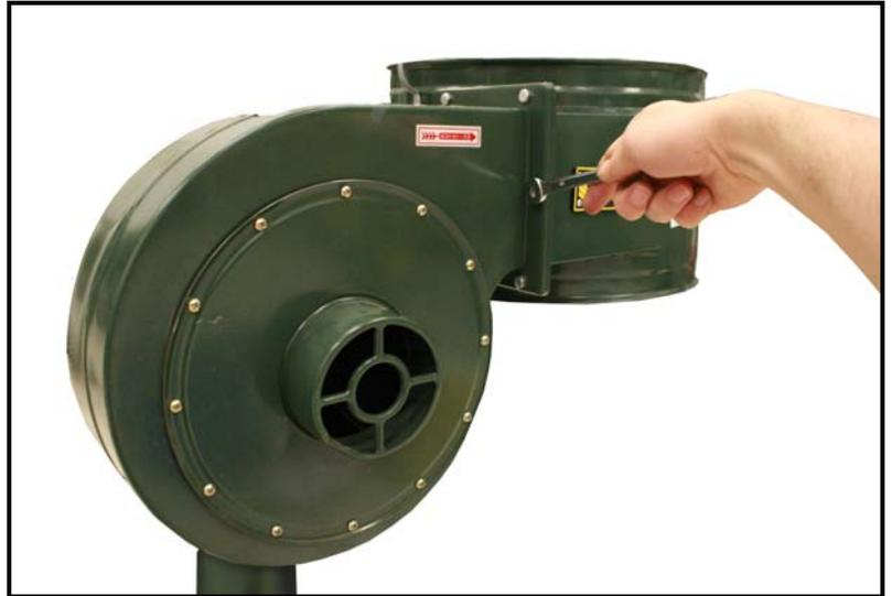
*Attaching Collector to the Motor/Impeller*
