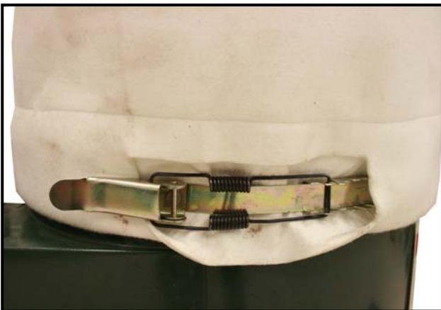
*Top Filter Bag Attached to the Collector*
