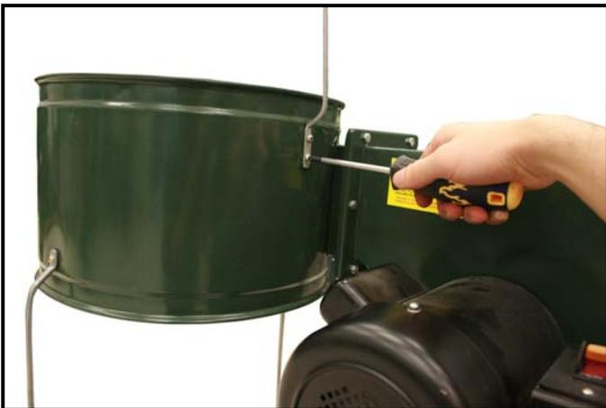
*Attaching Top Bag Support Bar to the Collector*
