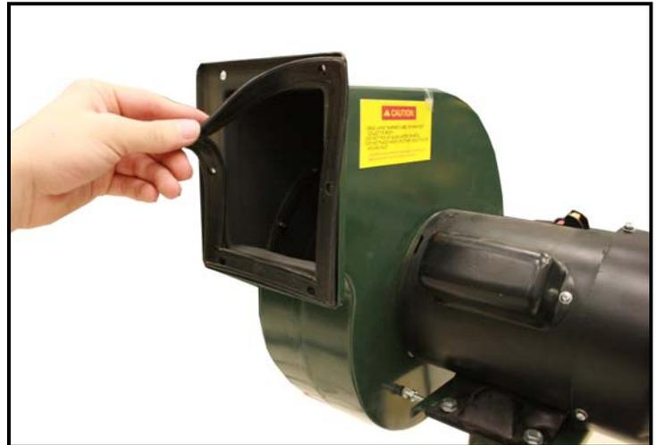
*Attaching the Gasket to the Impeller Opening*
