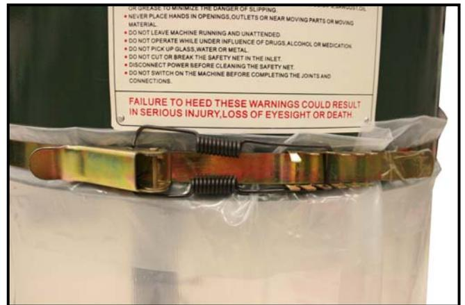
*Bottom Bag Attached to the Collector*
