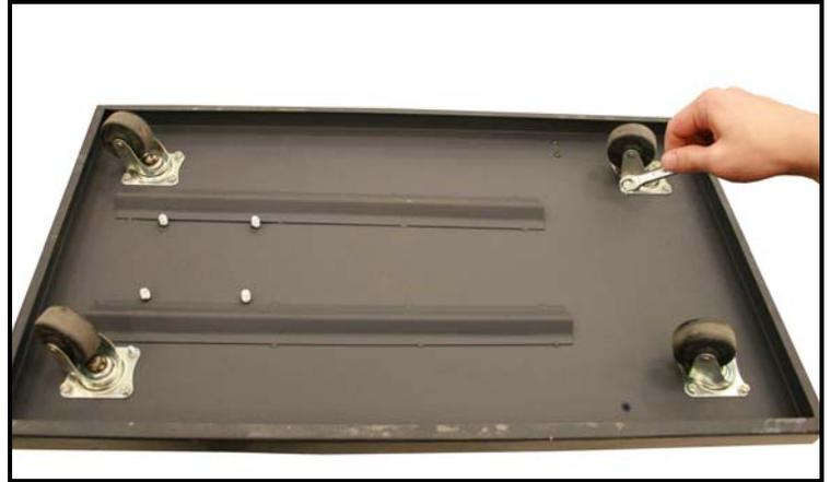
*Installing the Caster Wheels to the Base*
