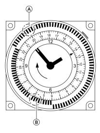
Push the switch relay contacts outwards for times when heating is required.
