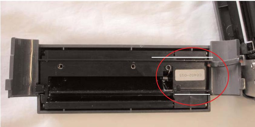
Figure 4. Wires are in between the 2 protruding sides of black bar.
