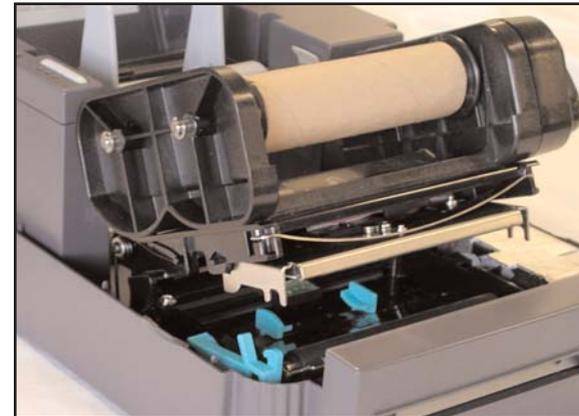
Figure 2. Ribbon Mechanism in open position with a core applied to the Ribbon Rewind Spindle.
