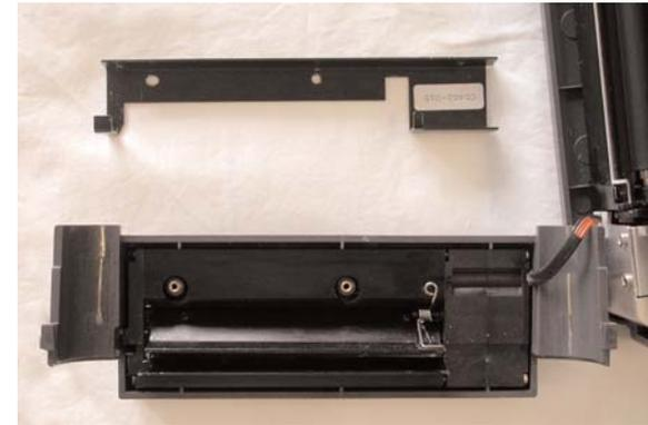
Figure 5. Black bar lifted off the cutter.
