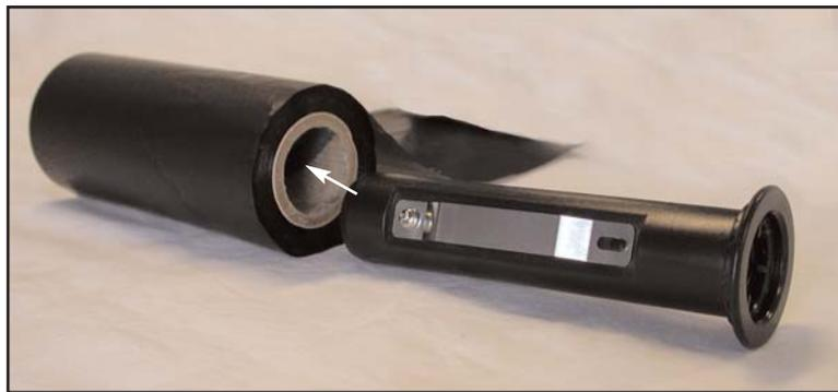
**Figure 4.** Step 3 Loading of Ribbon Supply on the Ribbon Supply Spindle. White arrow demonstrates which end of the Ribbon Supply Spindle is inserted into the Ribbon Supply.
