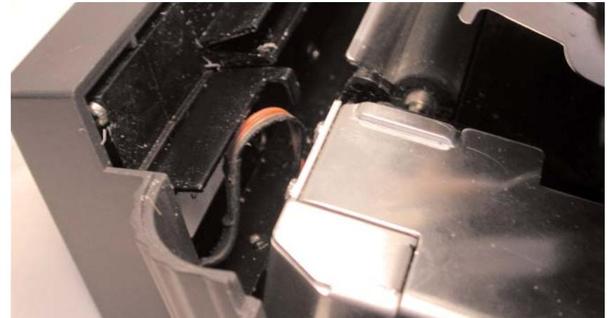
Figure 5. Wires are in between the 2 protruding lips of the black bar.
