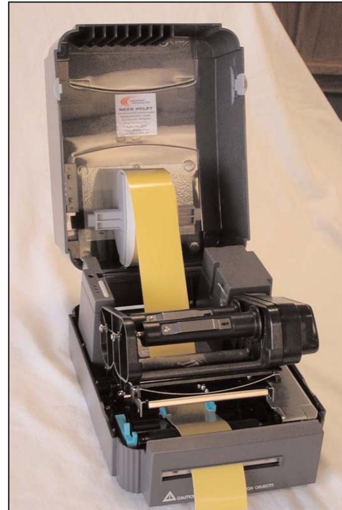
Figure 11. Label Media resting on the cover to allow more room during loading.
