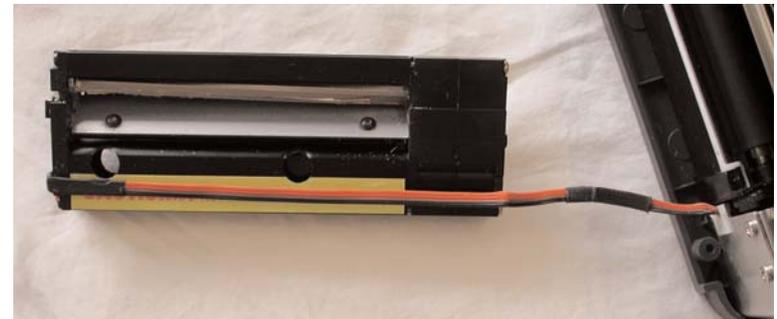
Figure 2. Wires correctly in front of the cutter.
