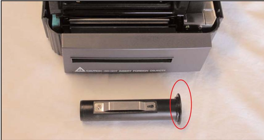
**Figure 3.** Flange of the Spindle should be on the right-hand side of the machine as demonstrated above.
