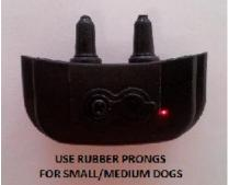
4) Test the shock of the collars by using the wire shock tester. Wrap the wires around the 2 metal posts of the collar then press the shock button. The bulb will light up if the collar is giving a shock.
