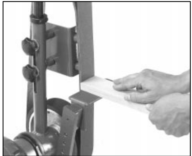
Figure 16. Belt sanding wood.
