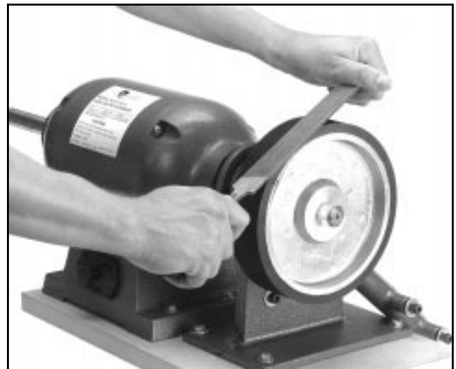
Figure 15. Relieving edges of drive wheel.
