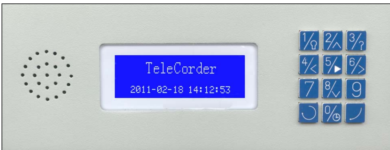
TeleCorder front view, showing speaker, LCD display and keypad.
