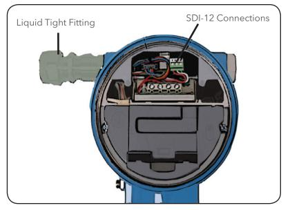
silicone or other sealant to prevent moisture from entering the Radar enclosure via the conduit piping. The thermal mass of the casting will cause water vapor to internally condense and accumulate with changes in the weather.
