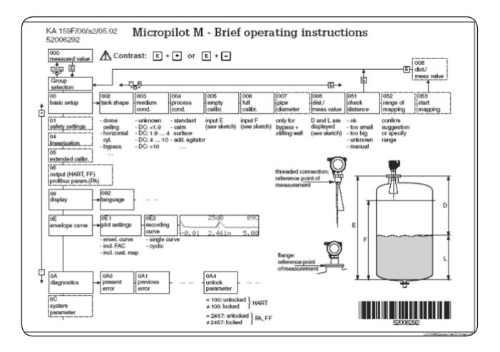
The radar unit supports other configurations such as tank volume gauging which are not used for stream gauging applications. When using the LCD setup menus, be careful to not indiscriminately alter the setup parameters. For special applications or problematic installations such as having false echoes from a bridge pier please contact WaterLOG for advice.
