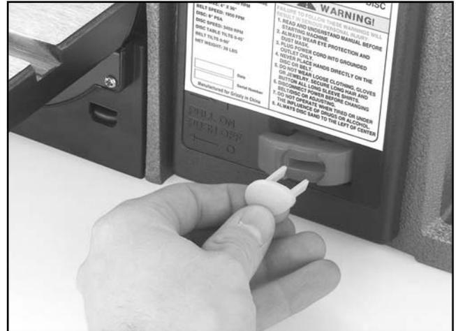
**Figure 16.** Inserting the safety key.
