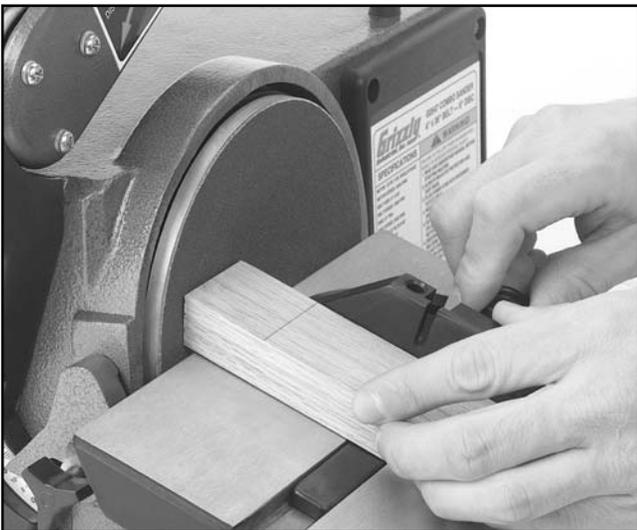
**Figure 19.** Mitering with the table angled.
