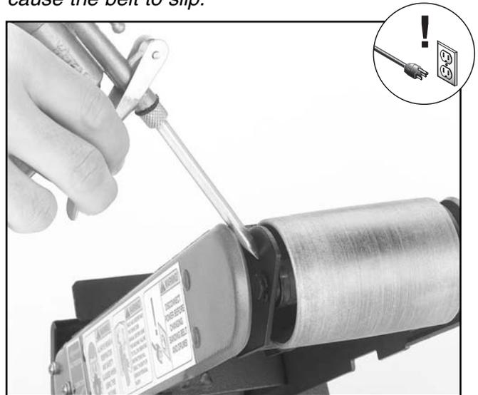
**Figure 25.** Lubricating the sleeve bearings.
