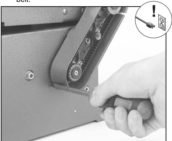
**Figure 24.** Tensioning the drive belt.
