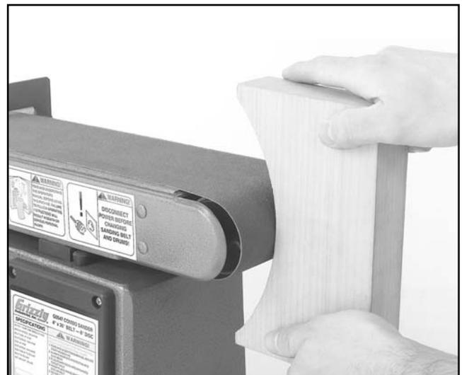
**Figure 22.** Sanding an inside curve.
