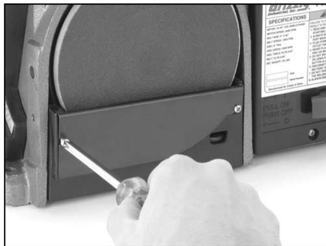
**Figure 4.** Attaching the disc guard.
