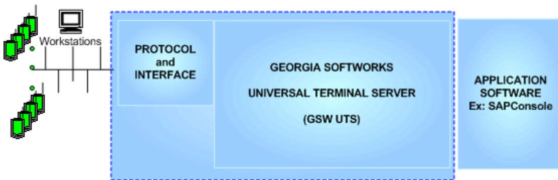
Figure 1: GSW Server Products Block Diagram
