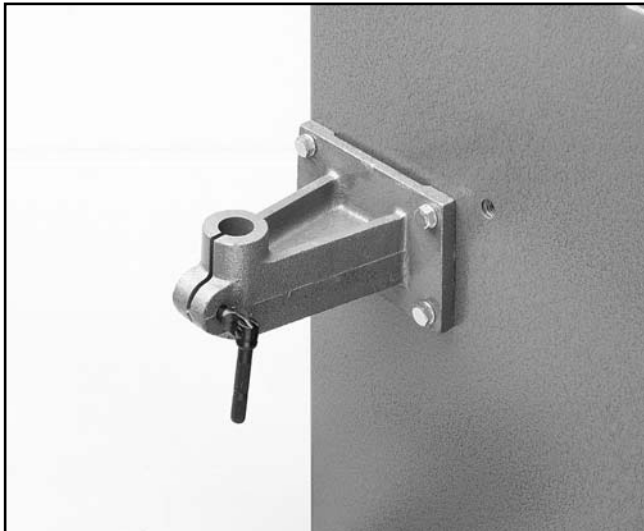
Figure 4. Lead screw bracket Installed.
