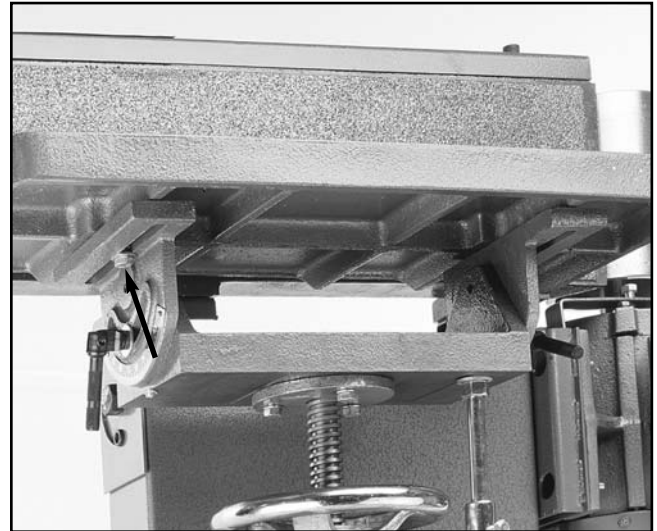
Figure 10. Attaching the working table.
