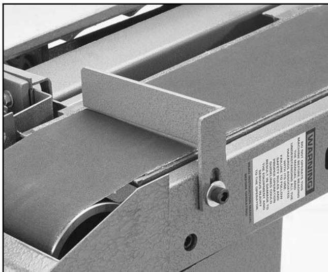
Figure 16. Back stop properly installed.
