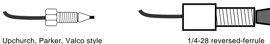
Figure 3-2. Note the direction of the ferrules: normal for Upchurch, Parker, & Valco; reversed for low-pressure 1/4-28.
