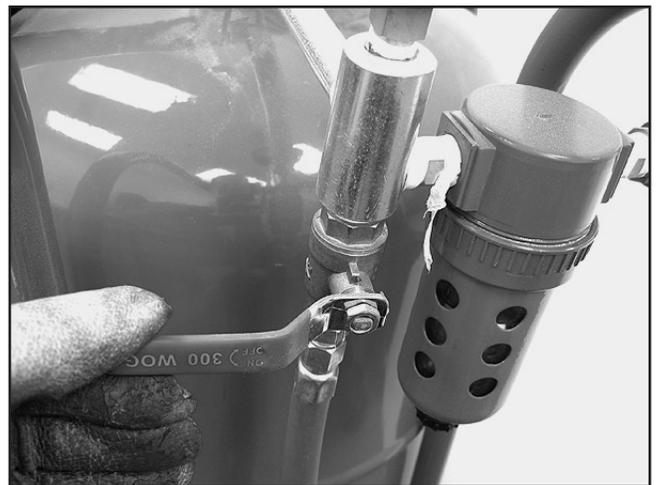
**Figure 9.** Blast hose air supply valve, closed.
