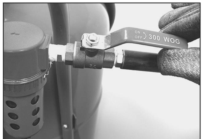
**Figure 12.** Tank air supply valve, opened.
