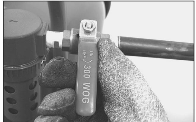
**Figure 8.** Tank air supply valve, closed.
