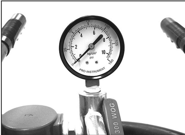
**Figure 10.** Tank air pressure at zero PSI.
