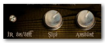
The factory setting for "Desert Voice Refurbished" comes with a convolution Impulse Response (IR) reverb already loaded. The IR can be disabled with the IR on/off button. The size and amount of reverb can be adjusted with the two dials...
